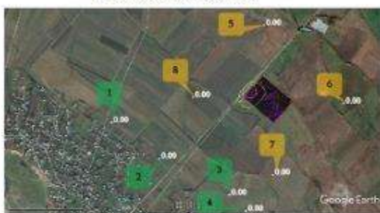
Maximum concentration of sulphur dioxide (code 330) at control points (nos. 1-4), at the nearest settlements and at the border of 500-m radii zone (nos. 5-8).
