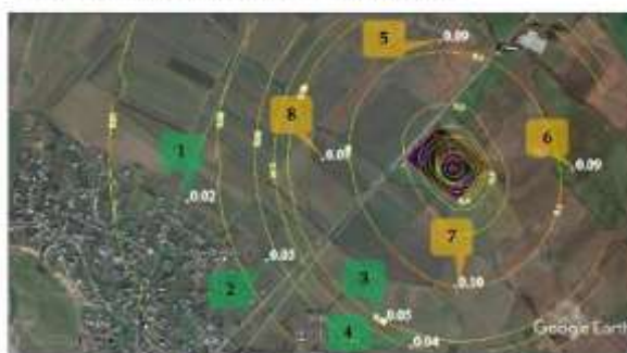
Maximum concentration of inorganic dust (code 2908) at control points (nos. 1-4), at the nearest settlements and at the border of 500-m radii zone (nos. 5-8).
